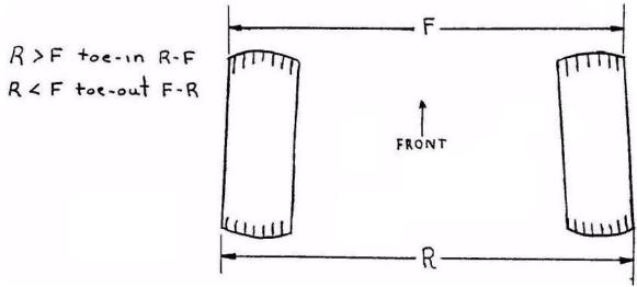
Consider the condition when your rear wheels are toed out ½". For every 24 miles you drive the wheels try to move sideways ¼ mile, each in the opposite direction. Thus the wheels are dragged sideways. This results in poor handling and rapid tire wear.
