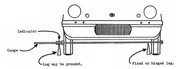
Gauge is shown in front of the front wheels, clearance will be less towards the center of the car and it may be necessary to remove the legs to lower the gauge. It is important that the gauge be at the same height in front and behind the axel, so use the same modified legs for ALL READINGS.
