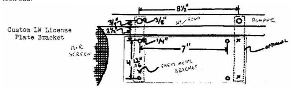
For the optional second bracket it will be necessary to drill holes in the plate.
