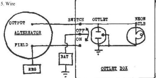
Note: Neon bulb lights up when 110v is available but remains off when using system for welding.
