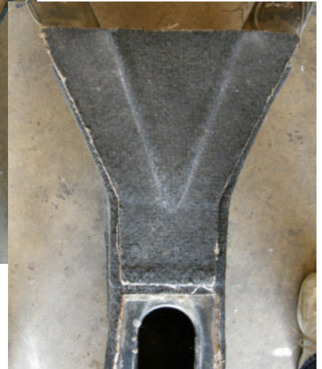
Top 'Y' piece, two pieces of jute bonded 0.25" + 0.50" thick
