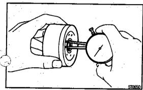
(b) Using a caliper gauge, measure the inside diameter of the center bearing.
