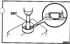
(c) Align the hollow of the internal gear with the protrusion is side the shock absorber, and remove the internal geal.
