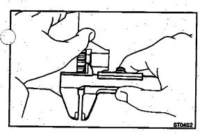
(b) Move the pinion gear toward the armature to remove slack and measure the clearance between the pinion gear end and stop collar.
