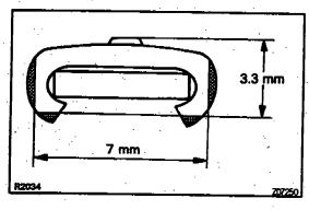
(d) Solder the pressed part, and shave to the specified in sures with the sandpaper etc.
