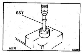
(b) Using SST and a press in a new center bearing to the position shown in the illustration.
