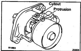
(d) Align the protrusion of the shock absorber with the cutout of the starter housing and install them.
