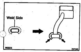
(c) Press the plate of the supply brush on the welded side the terminal lead wire.
