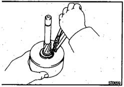
(g) Using snap ring pliers, install the plate washer and snap ring.
