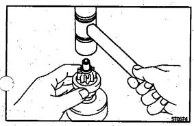
(e) Hold the starter clutch, tap the planetary shaft and instal the stop collar onto the snap ring with a plastic-faced hammer.
