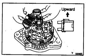
(b) Place the IC regulator together with the brush holder hoffzontally on the rectifier end frame.
