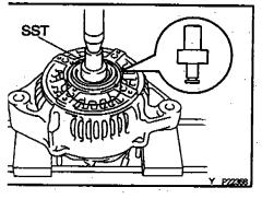
(b) Using SST and a press, press out the bearing. SST 09950-60010 (09951-00260, 09952-06010)
