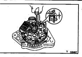
(c) Install the 5 screws until there is a clearance of approx. 1 mm (0.04 in.) between the brush holder and connector. Torque: 1.96 N-m (20 kgf-cm, 18 in.-lbf)
