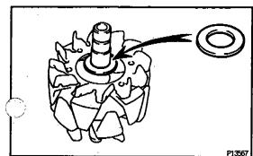
(c) Place the bearing cover (inside) on the rotor.
