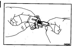
(c) Solder the brush wire to the brush holder at specified exposed length.
