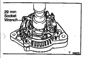
(b) Using a 29 mm socket wrench and press, slowly press in the rectifier end frame.
