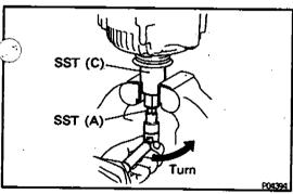
(e) To loosen the pulley nut, turn SST (A) in the direction shown in the illustration.
