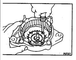
2. IF NECESSARY, REPLACE FRONT BEARING
