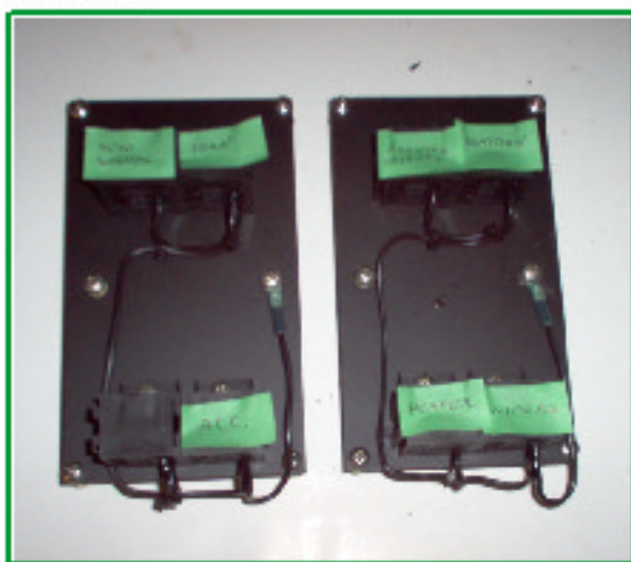
Relay panel, painted with grounded sockets.
