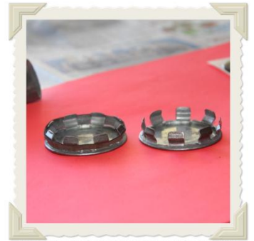
Band installed on prongs to provide snugness.
