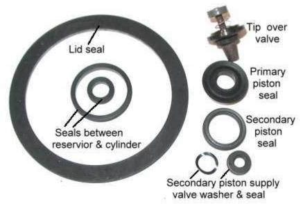
The seal on the primary piston is sometimes difficult to install. I coated the seal with grease and slipped it on over the pointed end. The correct orientation is with the largest part of the seal to the inside of the cylinder (the pointed end of the piston) as shown being installed in the top photo on the right. As you see, a small screwdriver helps. Caution, the seal will tear if stretched only slightly more than necessary to get it over the disk on the end of the piston.
