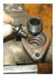
The next task is to remove the two pistons. With a little luck they'll come out when the cylinder is shook. However, we have other methods for the difficult ones. The scheme is to blow out the pistons with
