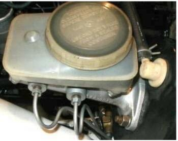
**Removing the PDWA:** The photo on right shows the PDWA on my '76 TR6. Before removing the PDWA I blow the fluid out of the system as described above. Next, I disconnect the electrical connector to the switch on the top and then disconnect the two pipes from the engine side of the PDWA and then remove the bolt securing the PDWA to the body. The PDWA will then lift off with the pipes that connect between
