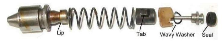
The next step is to put the secondary piston back together. I used the vise to squeeze the spring (I held the parts with one hand as shown in photo) and then used a small screwdriver in the other hand to push the thimble over the end of the piston and pressed the tab down behind the lip.
